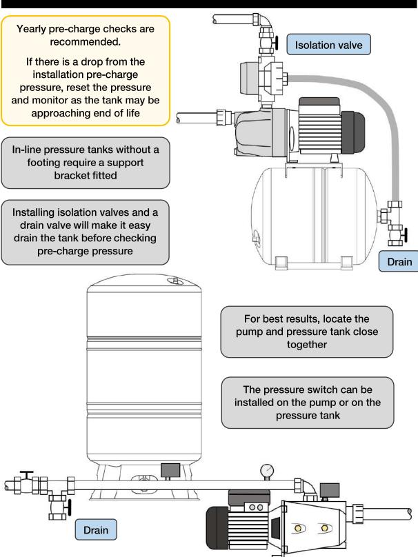
If there is a noticeable lag in water delivery, adjust the cut-in pressure upwards reducing the differential. Adjusting the cut in pressure does not require the tank pre-charge to be altered.
